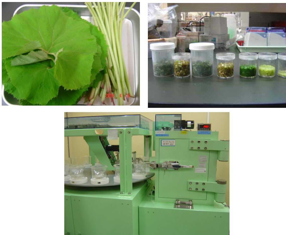
Figure 3. Giant butterbur leaf blade and petiole samples (left), cut plant tissue samples for Ge gamma spectrometry measurements (right), and the Ge detecting system with auto sampler (bottom).
