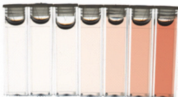
Fig.1 The color changes of the PVA-GTA-I dosimeter irradiated with mono-energy carbon beam; the dose levels were 0, 1, 2, 4, 10, 20, 40 Gy (left to right).
