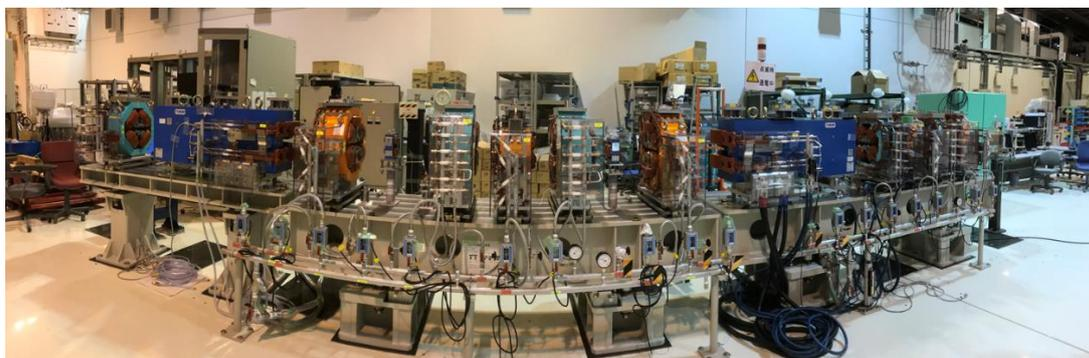
Fig. 2 Prototype of the half-cell of the 3 GeV storage ring
