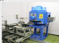
Response calibrator using 60 Co (SSDL in Japan)
