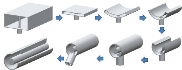
Fig. 2. Transformation from a coaxial-waveguide converter (top left) to a C-shaped waveguide (bottom left).
