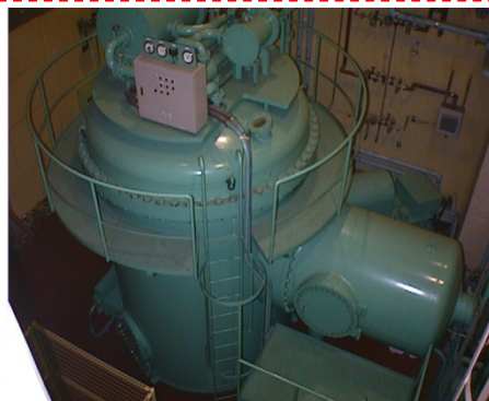
Electron accelerator (0.5~2.0 MeV 0.1~30 mA)
