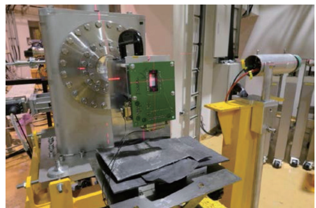
Figure 1. Device under test at PH1 during the alignment. A CCD is placed on the beam axis at room temperature and 1 atmosphere of pressure. Beam flux is measured with a scintillation counter prior to the experiment.
