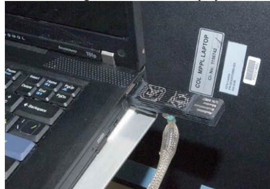
Figure 1. This shows one of the detector units attached to a USB port on one of the laptops onboard the ISS. This actual unit was calibrated at HIMAC.
