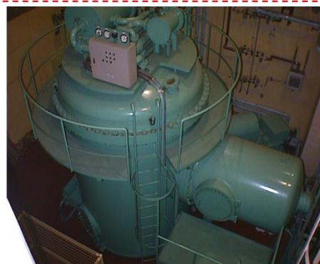
Electron accelerator (0.5~2.0 MeV 0.1~30 mA)
