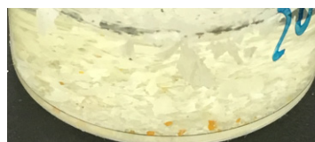
Fig. 2. Milky white and orange precipitate ( [\text{Pd(II)}]_{\text{ini}} : 1 mM, [\text{HNO}_3] : 0.1 M, [\text{TU}] : 0.1 M, 195 kGy, temp.: r.t.).
