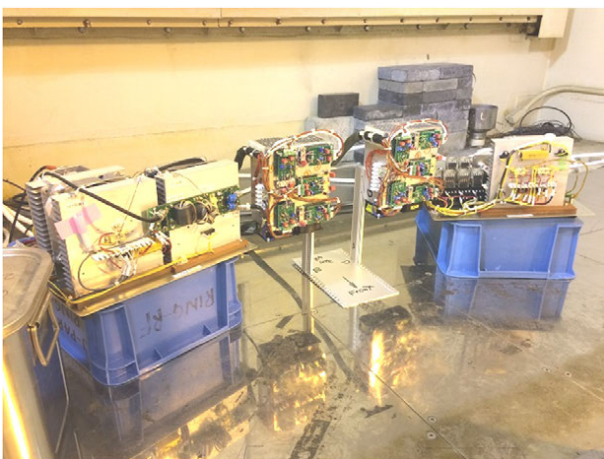
Fig. 1. The setup of irradiation test of solid state amplifier (left) at the QST. Middle and right show the setup to test MOSFETs without RF power.
