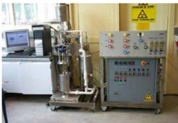
LIMETS 1 Tensile & Fracture toughness tests in LBE
