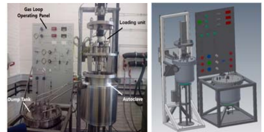
LIMETS 3 Fatigue tests in LBE
