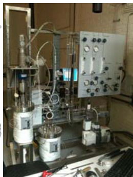
LIMETS 4 Tensile & Fracture toughness tests in LBE
