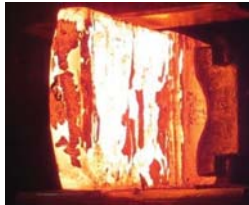
~ 6 ton ingot during forging
