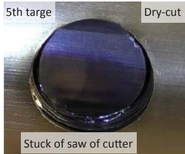
Inner most wall of 5th target remained window
