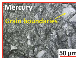
Fracture surface at 300 MPa
