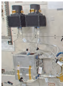
Fig.1 Photo for the preflight model of the PS-TEPC inside the Japan Experimental Module (JEM) of the International Space Station. It consists of two detector units (upper side) and a control unit (lower side).
