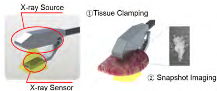
Figure 1. Conceptual diagram of the proposed hand-held endoscope-type x-ray imaging device.
