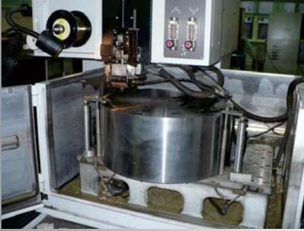
Wire-EDM machining of cylindrical S-65 beryllium block
