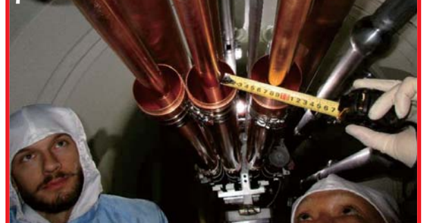
Transmission line assembly: Multiple high-voltage conductors are mounted in the pressure vessel
