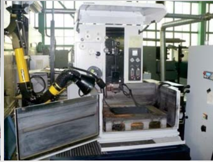
Wire-EDM machining of cylindrical S-65 beryllium block
