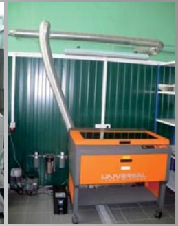
Laser marking of the tiles
