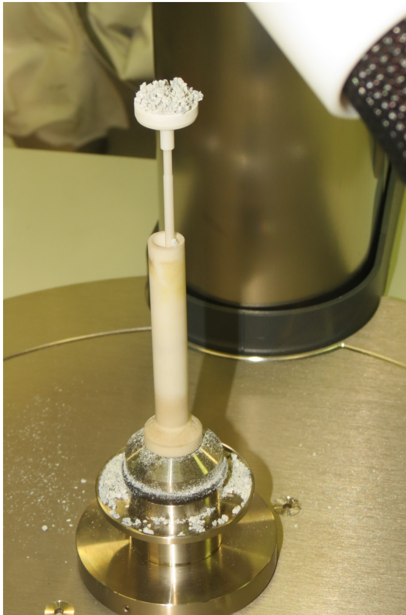
Fig. 3.9: Standard alumina crucible filled with beryllium pebbles (Lot 1843) after testing at 800 °C
