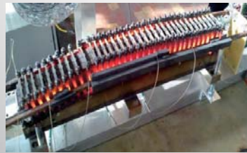
Inductive heating of the mockup with clamping tools
