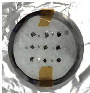
Hemisphere of pebbles embedded in the resin.
