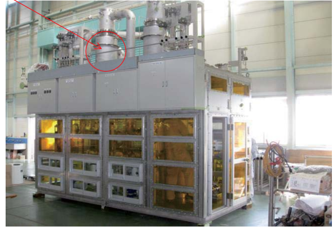
Pilot scale experimental apparatus for qualification of detritiation performance of scrubber column
