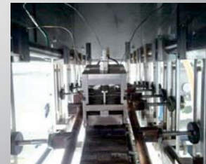
The mockup with modified clamping tools (in brazing chamber)
