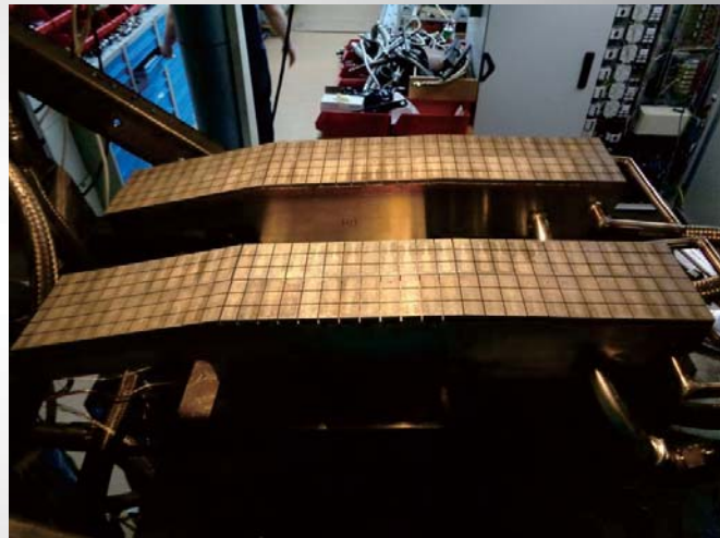
Two pair of PFU's installed in HHF testing facility
