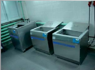
Ultrasonic cleaning of the tiles: Bath №1 – Ultrasonic bath Bath №2 – Rinsing in distilled water with stirring Bath №3 – Hot-air drying
