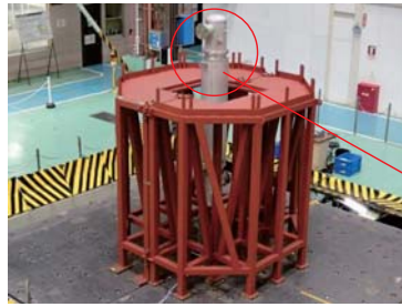
Scrubber column on 3D shaking table
