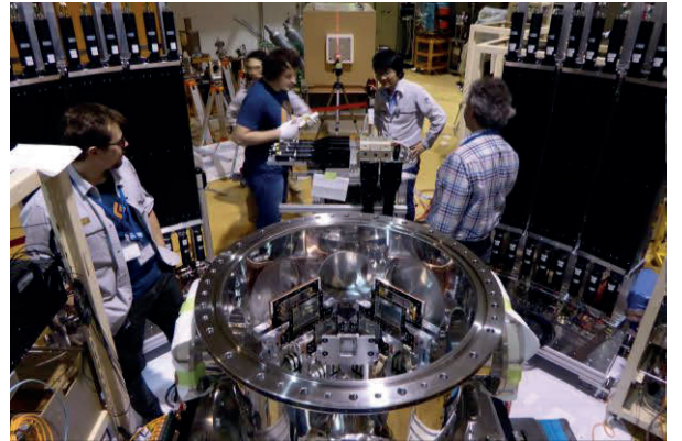
Figure 1: Setup consisting of target, three layers of silicon detectors, TOF detectors and dE-E detectors in downstream direction
