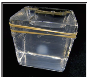
Fig. 1 A photograph of the polymer gel dosimeter irradiated with C ion (290 MeV/u) from four directions. The sample was prepared by putting gel sheets on top of another in the glass vessel.
