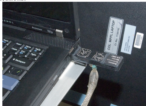
Figure 1. This shows one of the detector units attached to a USB port on one of the laptops onboard the ISS. This actual unit was calibrated at HIMAC.
