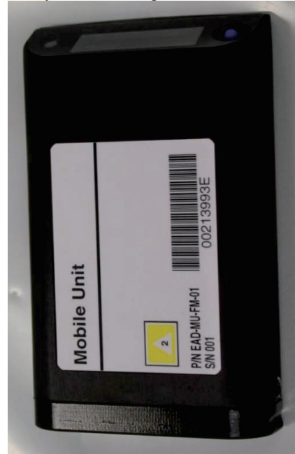
Figure 4: Active personal dosimeter final calibrated and ready for the flight to the ISS
