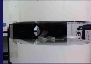
0.3T MRI with hole in yoke
