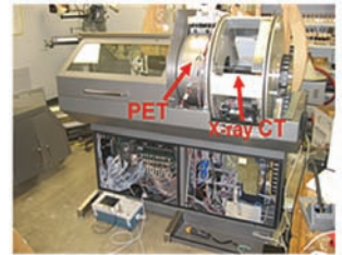
Figure 2. A picture of the MuPET gantry.
