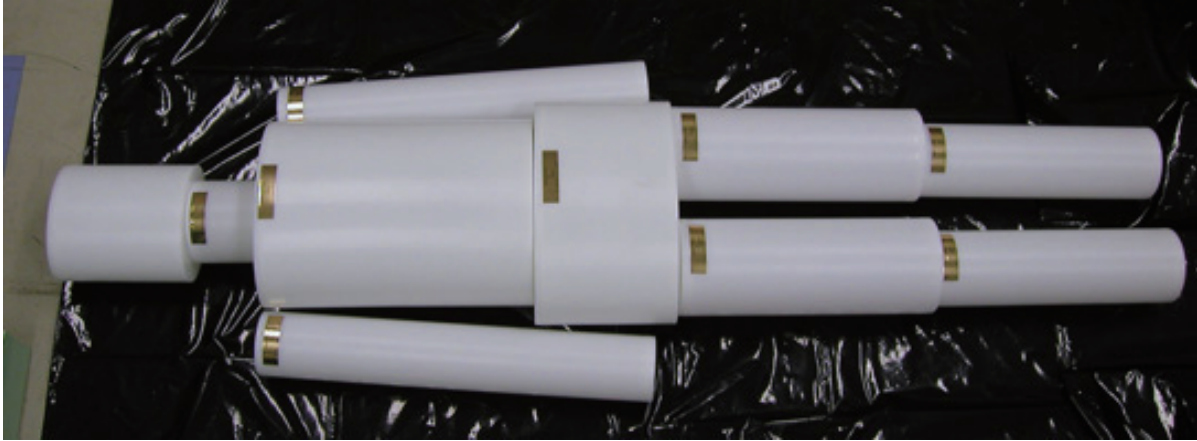
Figure 5. Exterior of the BOMAB phantom used for the calibration 3)
