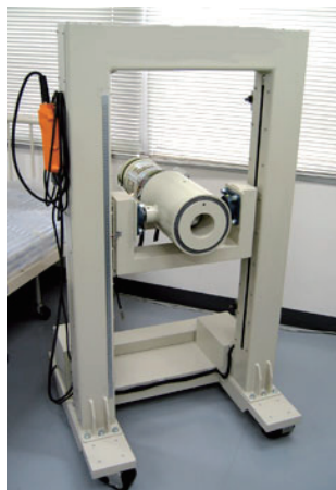
Figure 1. System for thyroid counting
