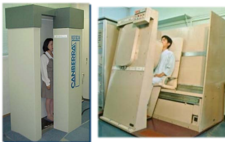
Figure 1. Picture of the WBCs used in this work (left, stand-up geometry; right, chair geometry).
