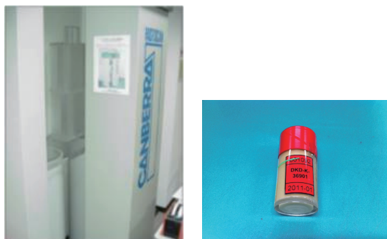
Figure 2. Canberra Transfer Phantom (CTP) and the calibration source
