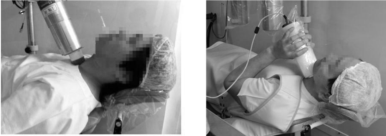
Figure 2. Thyroid counting with a HPGe detector (left) and a NaI(Tl) detector (right)
