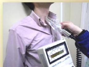
applied NaI(Tl) scintillation survey meter as substitution
