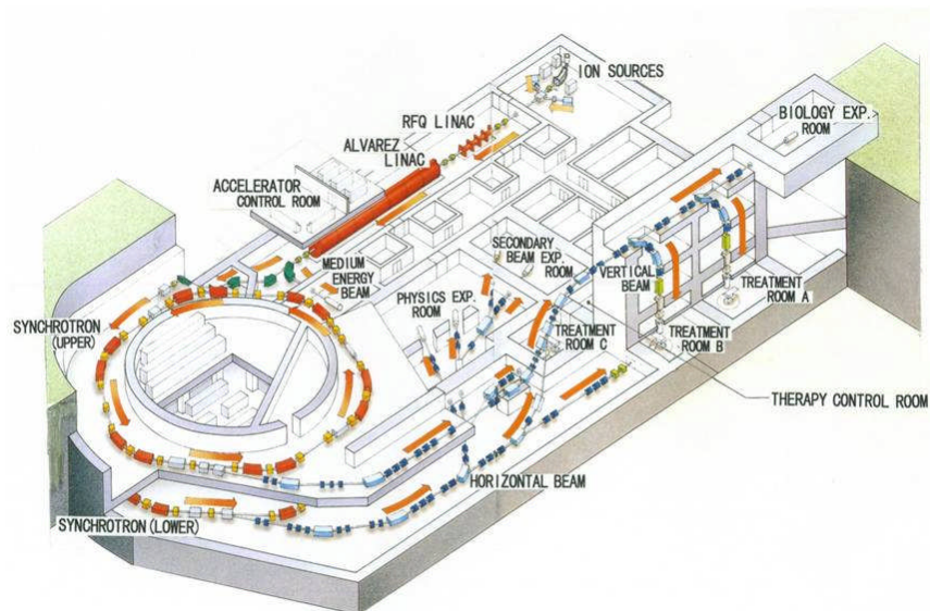
Fig.1 Cut-away view of the HIMAC facility
