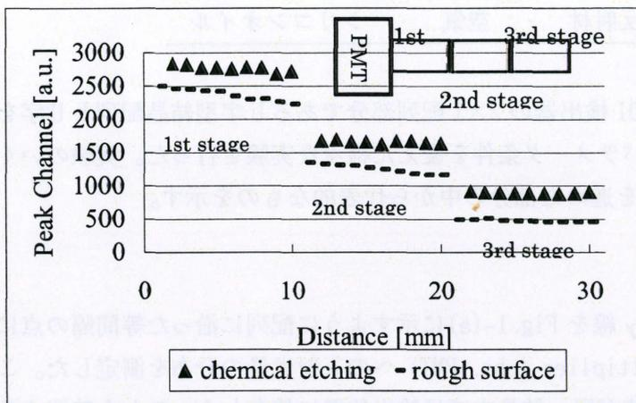
Fig.2 Position dependence in each crystal element.
