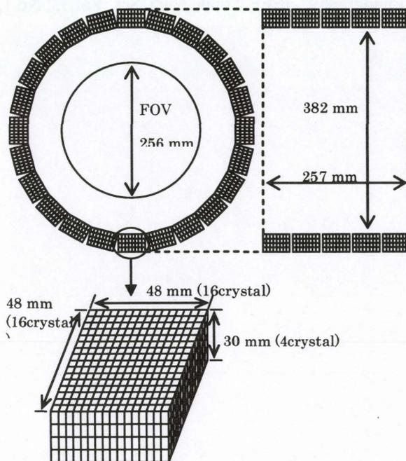
Fig. 1 Design of the next generation PET scanner.
