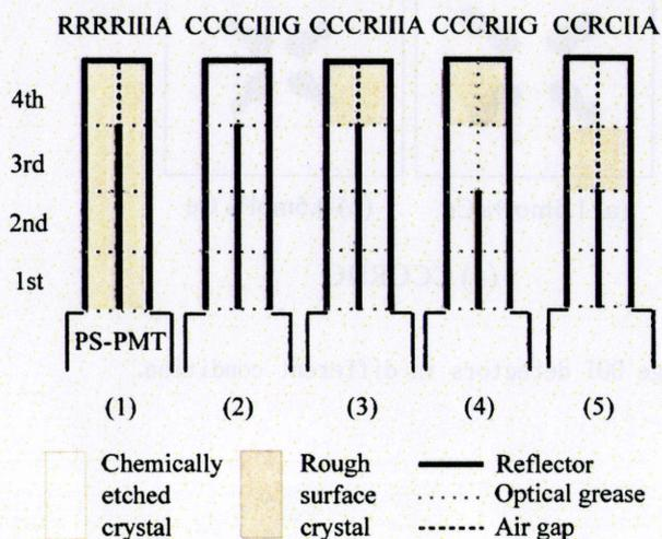
Fig.1 Structure of 4-stage DOI detectors for experiment.
