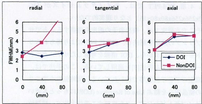
Fig. 4 Resolution of the reconstructed images
