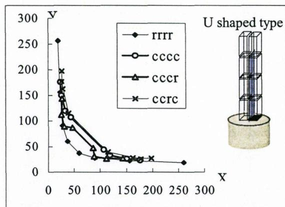
Fig.4 Full energy pulse heights of each crystal element in U shaped array with reflector in 1st, 2nd, and 3rd stage.
