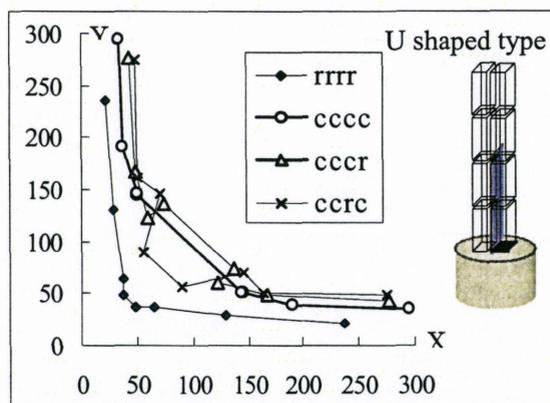
Fig.5 Full energy pulse heights of each crystal element in U shaped array with reflector in 1st and 2nd stage.
