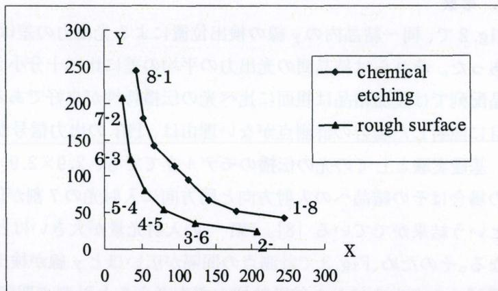
Fig.3 Full energy pulse heights of each crystal element having rough or chemically etched surface in straight line array.
