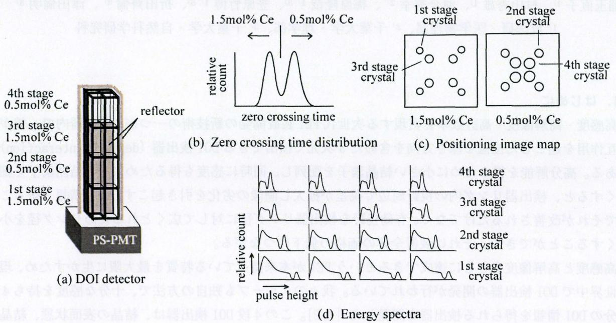
Fig.1 (a) Design of a 4-stage DOI detector and conceptual drawings of (b) zero crossing time distribution, (c) positioning image maps, and (d) energy spectra.
