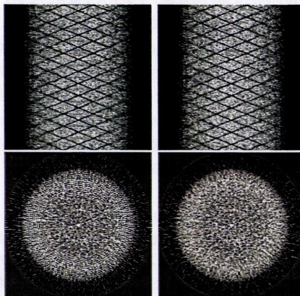
Fig. 3 Rebinned sinogram and reconstruction image.
