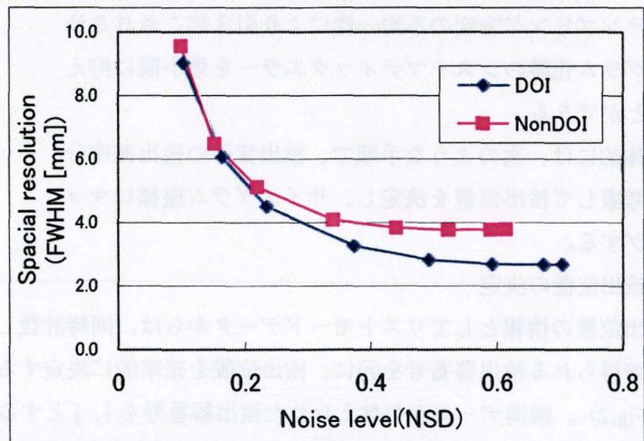
Fig. 5 Graph showing trade-off between special resolution and noise standard deviation (NSD)
