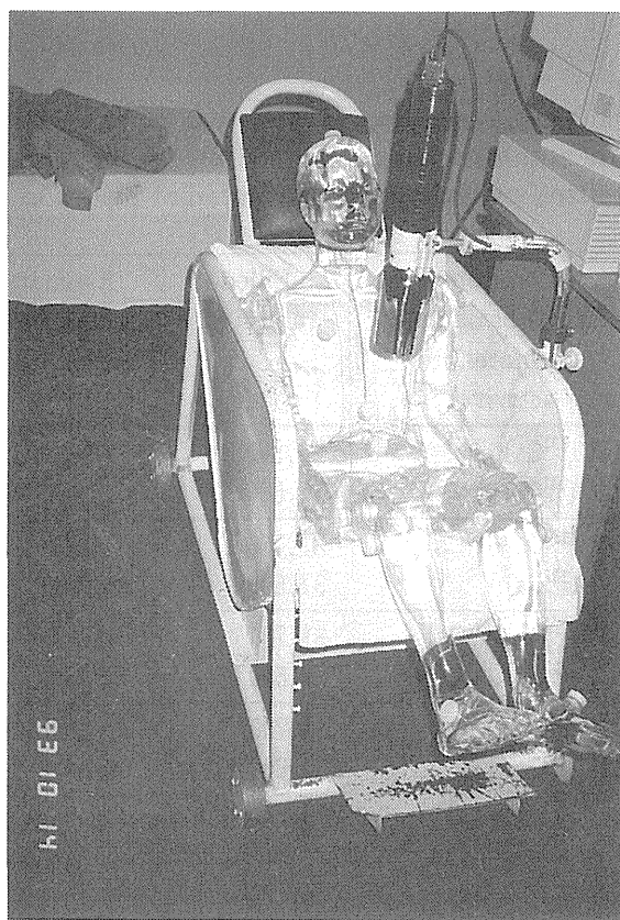
Photo.5 Anthropometric phantom measurement by the portable whole-body counter in Mother and Child Polyclinic in Ukraine in 1993
