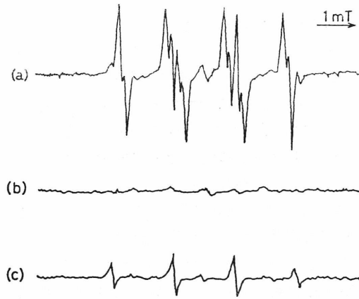
Fig. 1. ESR spectra obtained from the hypoxanthine (HPX)-xanthine oxidase (XOD) system in the presence of DMPO. Reaction mixtures contained 0.5 mM HPX, 0.1 unit/ml XOD, 125 mM DMPO, and no addition (a); 0.025 mM Cu(II)(CyHH) 2 (b); 0.25 mM Cu(II)(CyHH) 2 (c).
