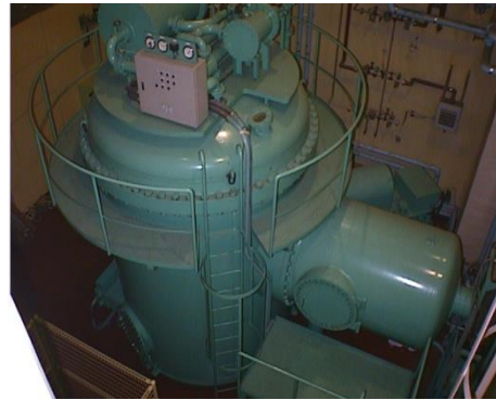
Electron accelerator (0.5~2.0 MeV, 0.1~30 mA)
