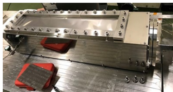
Fig. 1. Photograph of manufactured electron beam irradiation vessel.
