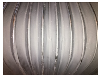
Fig. 3. Bellows after 450 strokes.
