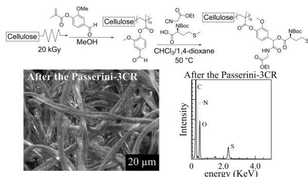
Fig. 1. SEM image and the corresponding SEM-EDX spectrum of the PMV after the Passerini-3CR with ethyl isocyanoacetate and N -Boc-L-methionine.
