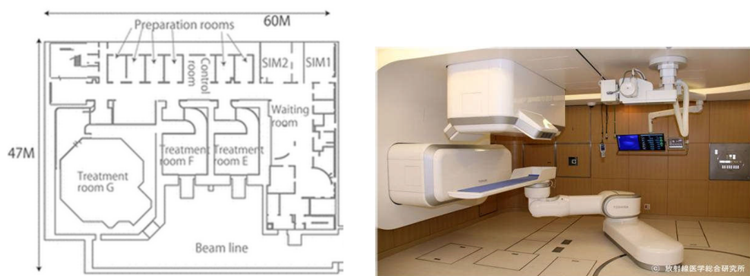
Fig. 2. Layout of the treatment floor in the new facility (left) and the treatment Room E, with two fixed beam ports and a SCARA-type robotic arm (right).
