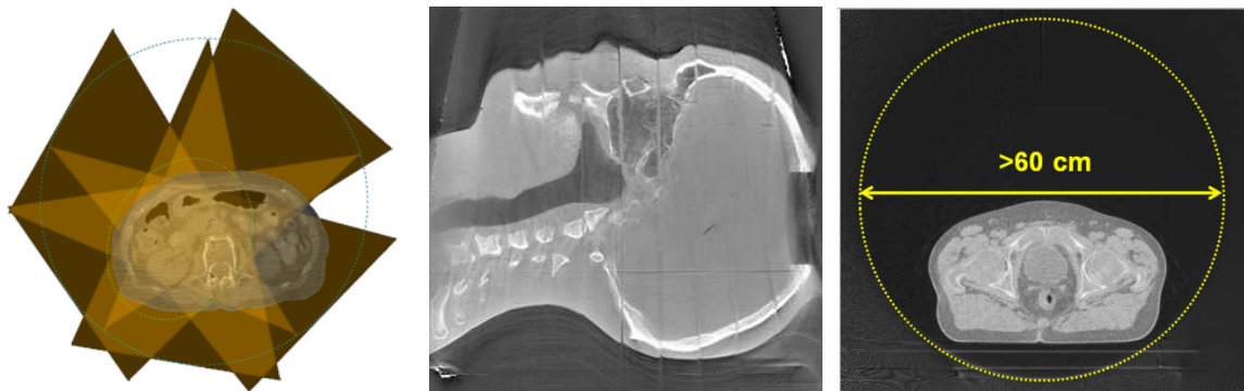
Figure 6: From left to right: Principle non-isocentric limited FOV CBCT, Sagittal short-scan CBCT and large FOV CBCT.
