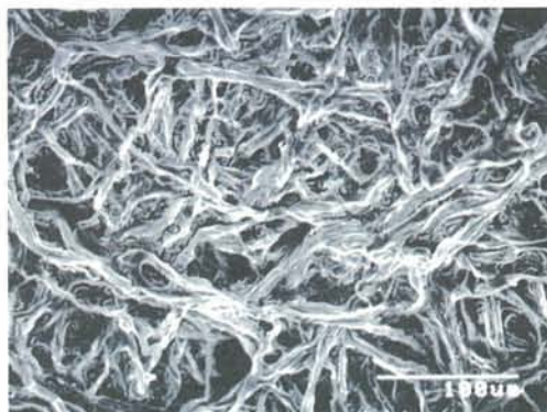
Photo 2 Electron microscope photograph of fibrous SiC ceramic
