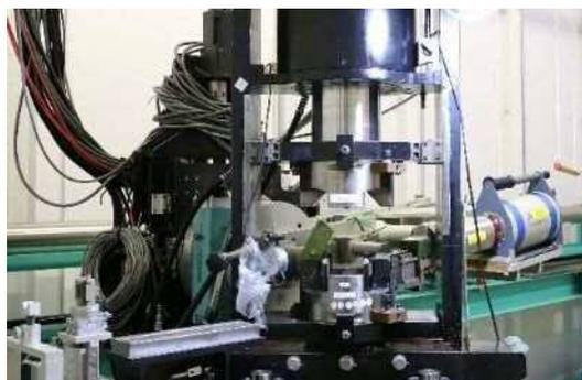
Fig. 1. Photograph of in situ synchrotron-radiation X-ray diffraction measurement system.
