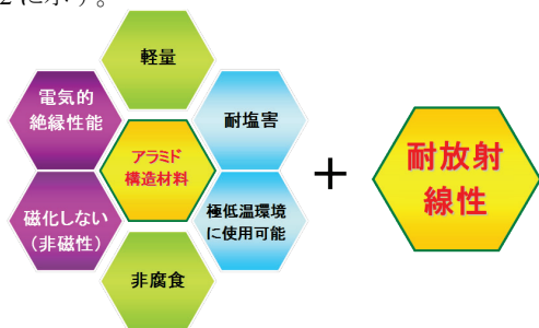
Fig. 2 Performance of new braided aramid fiber bar.
