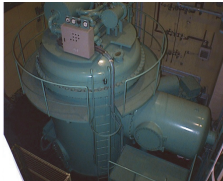
Electron accelerator (0.5~2.0 MeV 0.1~30 mA)
